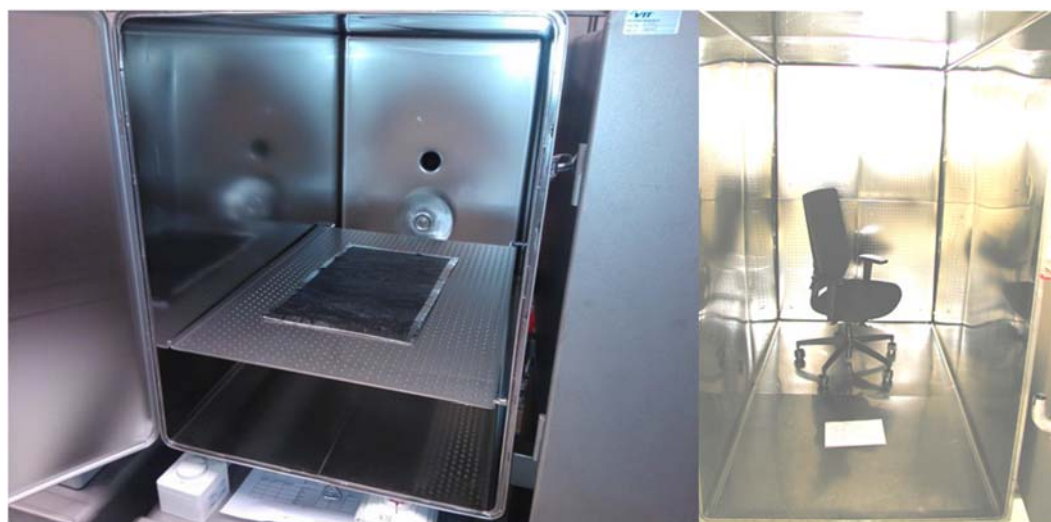
Picture 7 Emission measurement samples in chambers
